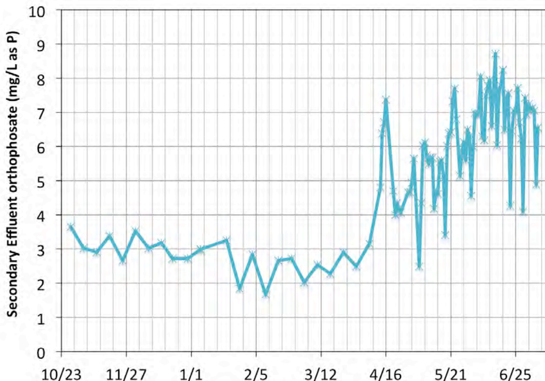
Figure 3.21 – Phosphate concentration in the secondary effluent during piloting (includes effect of CEPT control)
