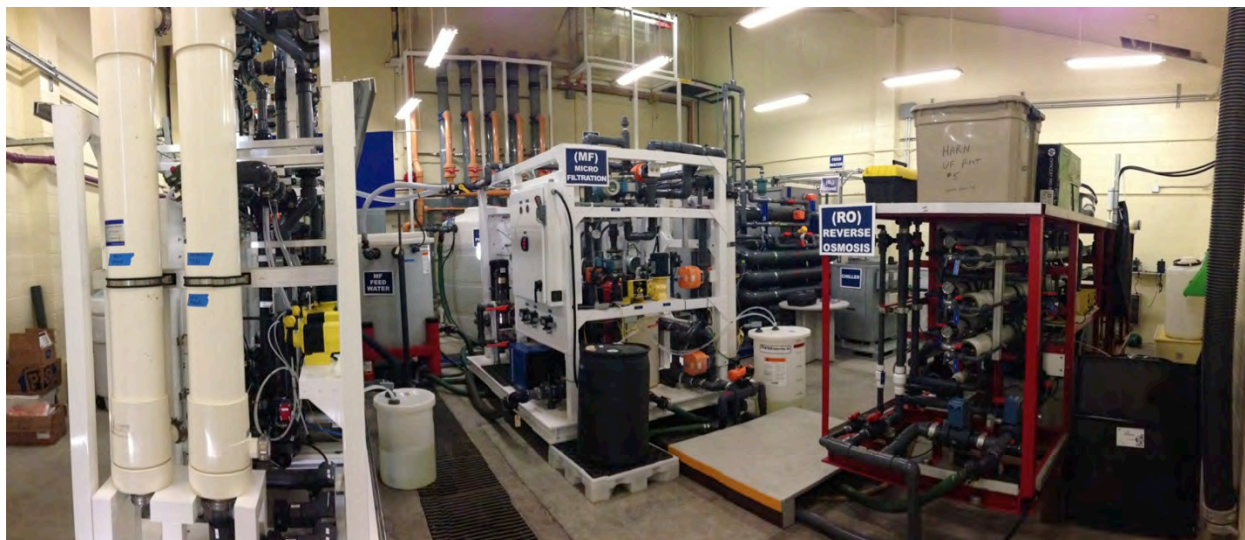
Figure 2.3 – Photo of pilot facilities. Outside-in MF front left; BAF equipment back left (not used); inside-out MF center; ozone back left; and RO right.
