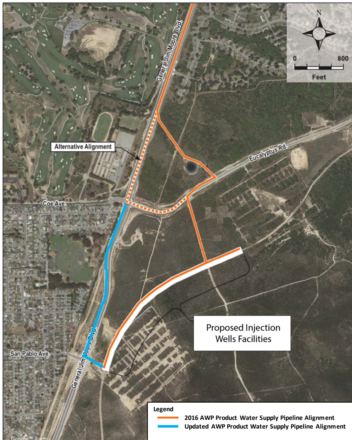
Figure 3-7. Map of AWP Facility Product Water Supply Pipeline to Proposed Injection Well Facilities
